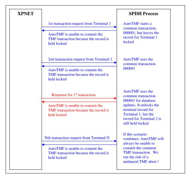
Fig. 5 – Device Handler processes leaving Records locked
