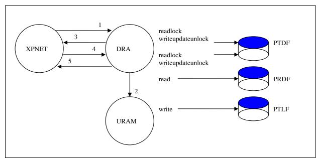
Fig. 4 – Example Message Flow (before AutoTMF)
