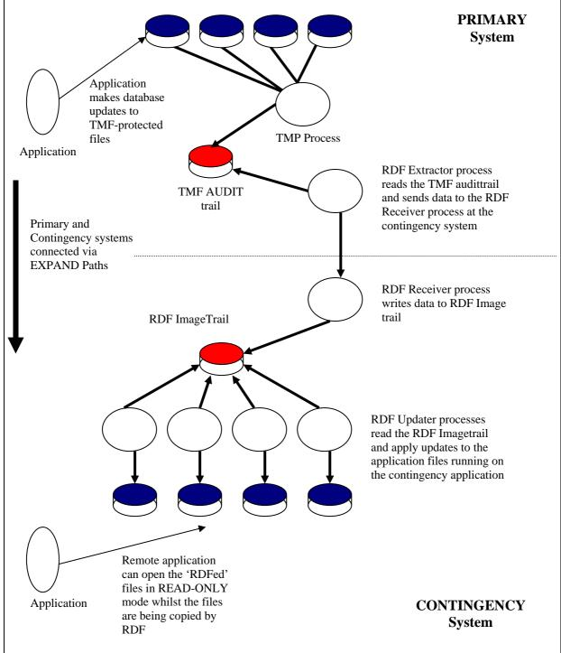
Fig. 6 - Basic RDF Systems Architecture
