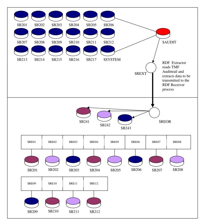
Fig. 8 - An Example TMF Configuration to support multiple BASE24 Logical Networks
