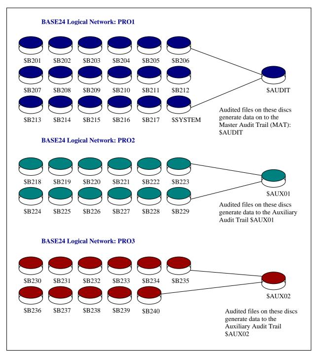
Fig. 7– An Example TMF Configuration to support multiple BASE24 Logical Networks
