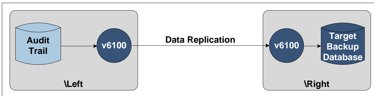
Figure 3 – Replicating Data from a Source Database to a Target Database
