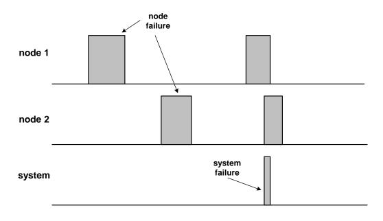
As shown in Figure 1, the active/active system fails only if more than the configured number of spare nodes fails (for instance, in a singly-spared system, a dual node failure is required to bring the application down).
