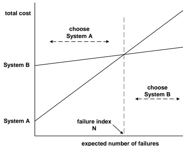
industry-standard server (ISS), and System B is a two-node cluster of industry-standard servers. For this example, let us assume the following initial costs and restore times from a single node failure:
